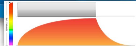
CW Laser Exposure: 100% Duty Cycle (DC)
